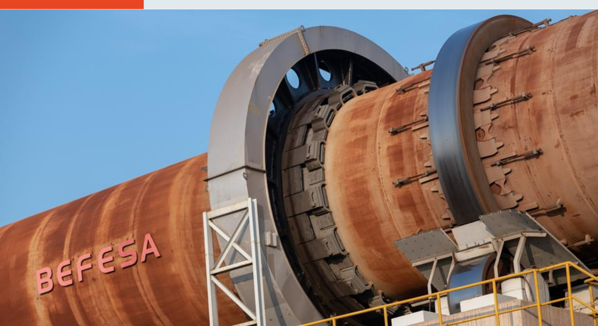
Waelz kiln at EAFD recycling plant in Gyeongju, South Korea
